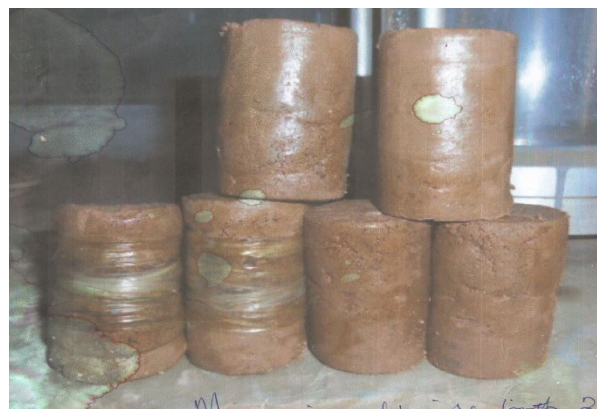
Figure 1: Typical Salt Compound and Test Specimen (Magnesium Chloride).
